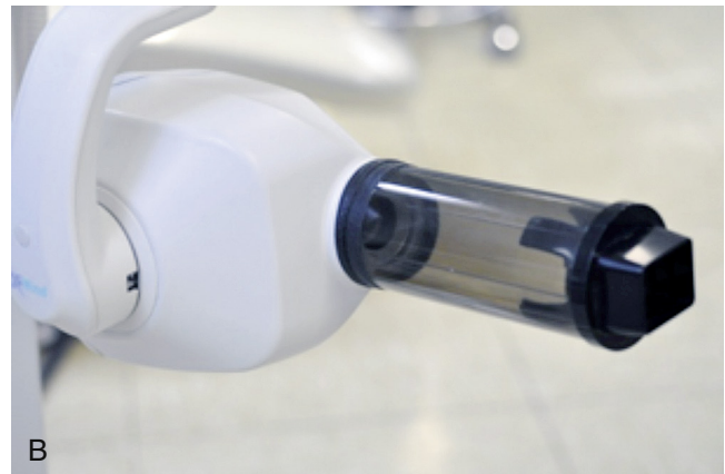
Fig. 2.2 Examples of rectangular collimators. The rectangular end of the beam-indicating device decreases the exposed surface by more than 50% compared with a 2.75-inch-diameter round collimation. (A) A non removable rectangular collimator mounted on an intraoral x-ray machine. (B) A removable rectangular collimator (DENTSPLY® Universal Collimator) mounted on the circular open-ended beam-indicating device.
