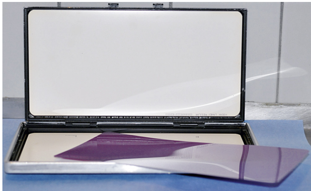
Fig. 2.4 An opened panoramic cassette (15 × 30 mm) with intensifying screens on both sides (white surfaces) and analog film (blue-purple). A similar cassette, but without intensifying screens, is used for phosphor storage plates.
