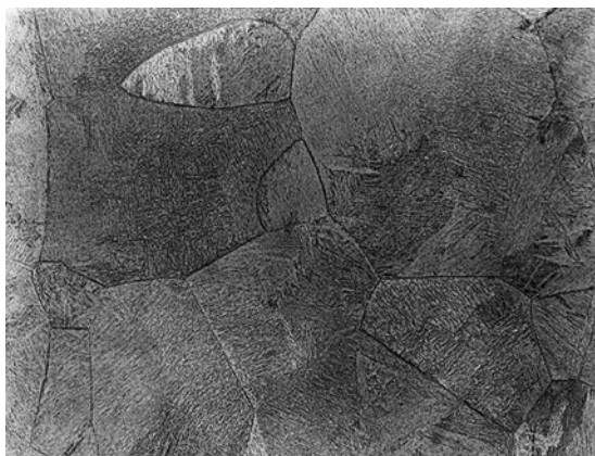
FIG. 10.12 Microstructure of as-cast Ti-6Al-4V.
