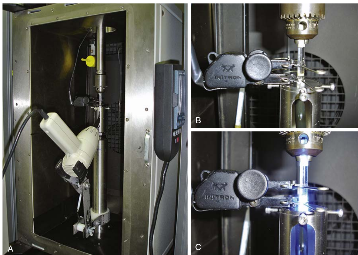
FIG. 5.19 Tensilometer for measuring polymerization stress during cure of composites. (A) Overview of test configuration. (B) Detail of test specimen and extensometer. (C) Detail as composite is photoactivated.
