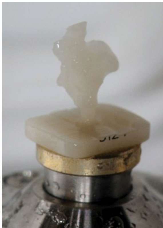
Figure 15.23 (F) Inlay restoration captured, still connected by the sprue pin to the CAD/CAM ceramic ingot.
