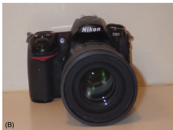
Figure 7.5 Examples of standard “point-and-shoot” (A) and single-lens reflex (SLR) (B) cameras. It can often be difficult to differentiate between the two; however, almost all point-and-shoot cameras do not allow for lenses to be removed and exchanged for other ones.
