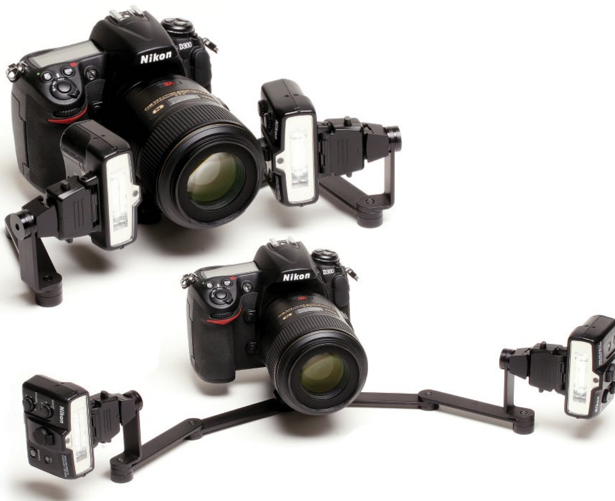
Figure 7.13 An example of a camera attachment which allows multiple positions for the macro flash. Moving the flash away from the lens makes it more difficult to control lighting, but it rewards the photographer with better shadows and highlights for diagnostic purposes.
