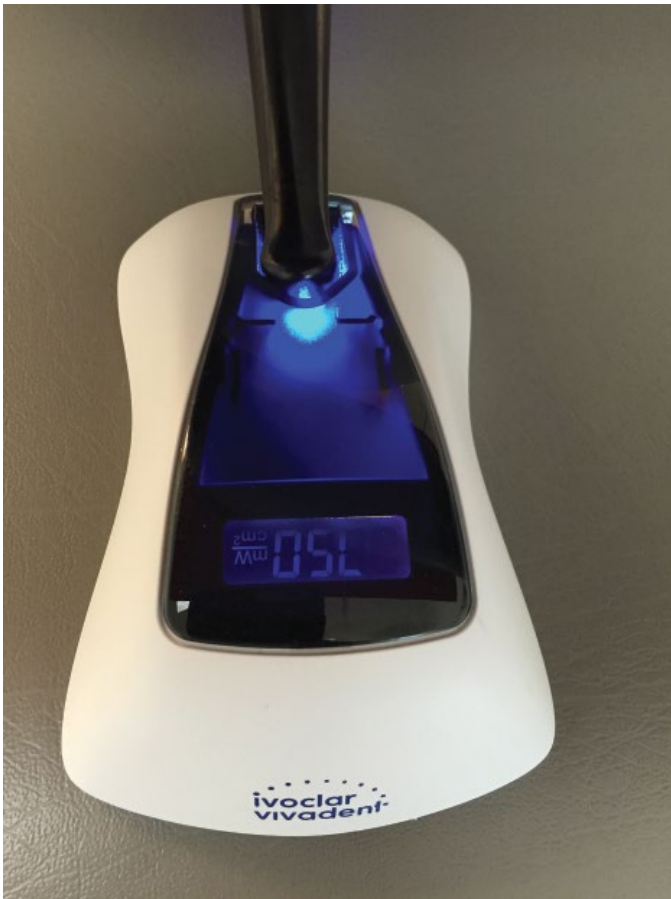
Figure 14.21 Light tips must be kept clean and your light source periodically checked with one of several diagnostic testing devices Bluephase Meter (Ivoclar Vivadent).
