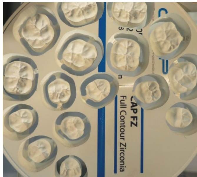
Figure 46.24 Crowns milled from a puck of CAP FZ (Custom Automated Prosthetics) full-contour zirconia. Source: Figure courtesy of Custom Automated Prosthetics.
