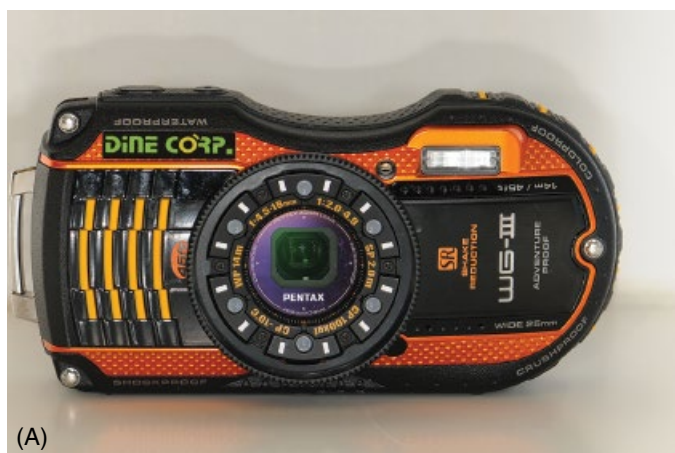
Figure 7.5 Examples of standard “point-and-shoot” (A) and single-lens reflex (SLR) (B) cameras. It can often be difficult to differentiate between the two; however, almost all point-and-shoot cameras do not allow for lenses to be removed and exchanged for other ones.
