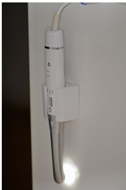
Figure 3.9 (A) This Kodak 1600 intraoral camera has auto focus which can either be wireless or wired, and it makes it easy for both dentist and hygienist to quickly record a patient's condition including potential caries identification technology.
