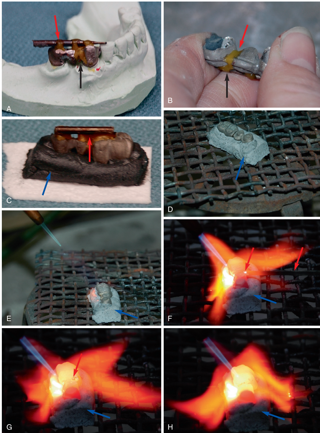
FIG 12-9 Soldering alloys. Sometimes, an alloy restoration must be cast in several pieces and then soldered together before cementation. In general, the pieces of the restoration are juxtaposed in the mouth and temporarily held together ("indexed") with sticky wax or a resin material. In these images, the juxtaposed pieces are shown on a master cast ( A ). The final desired shape of the solder joints are then waxed ( B ), followed by investment of the restoration into soldering investments ( blue arrows in C ). Once the investment has set, the wax and index are removed and the investment is placed onto a soldering stand ( D ); flux paste is generally added at this point. A small reducing flame is gradually applied to the investment and restoration ( E ), and then solder ( red arrows in F , G ) is added while maintaining the reducing atmosphere of the flame. Heating continues until the ball of solder ( red arrow in G ) flows into the solder joint ( H ). At this point the temperature of the castings is about 50 to 100° C below the melting point of the alloy, so the heat must be removed to prevent damage to the castings. It is significant to note that with all-ceramic restorations, soldering is not possible. (Courtesy M. Owens, C. S. Bemis, and D. E. Owens CDT, Georgia Regents University, Augusta, GA. Photography by R. Messer, Georgia Regents University, Augusta, GA.)
