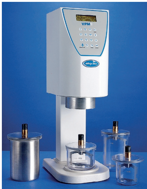
FIG 9-6 Programmable, power-driven vacuum mixing unit. The unit is designed for vacuum mixing all types of gypsums, plasters, and investments. Utilizing multiple stages, the VPM2 can be programmed for time, speed, and paddle direction. A twin-chamber, oil-less vacuum pump offers a powerful vacuum quickly, removes air, and reduces the risk of bubbles, providing a bubble-free mix. (Courtesy Whip Mix Corp, Louisville, KY.)
