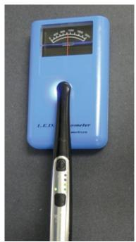
**FIGURE 40.3** Light-curing unit showing power output via a radiometer.
